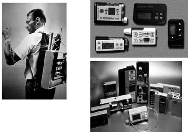
Figure 9 In 1974 Gérard Slama designed the first prototype for an intravenous insulin pump (left). First CSII system was used by John Pickup and Harry Keen, in 1978. Later on, pumps have been reduced in size and developed programs for multiple basal rates of insulin infusion and premeal bolus (right).
